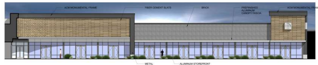
NORTHEAST BUILDING ELEVATION SCALE: 3/32" = 1'-0"
